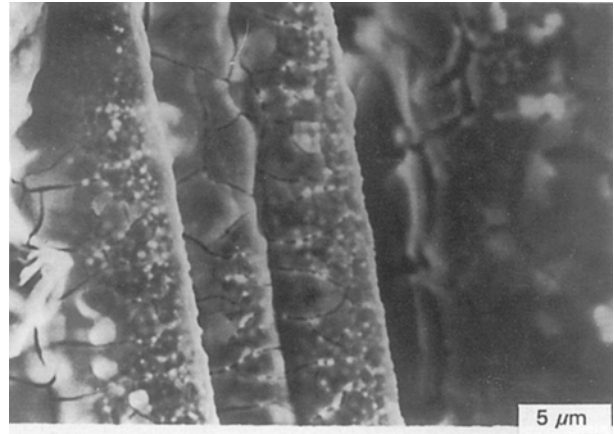
Figure 4 Cracking of the nickel coating with coating thickness > 1.0 \mu\text{m} for brominated fibres.
